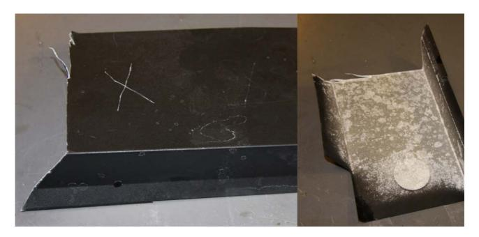
After 14 days of total exposure the metal roof plate is showing more degradation and now assumed red Iron oxides is present at the cutting edges and inner surfaces (red arrows).
