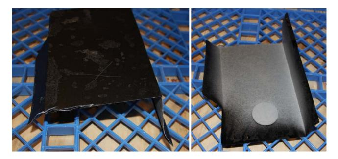
After 7 days of pre-exposure the inside coating is also showing signs of corrosion, metal oxides penetrating the coating is assumed to be Zinc oxides, there is no visible red Iron oxides present.
